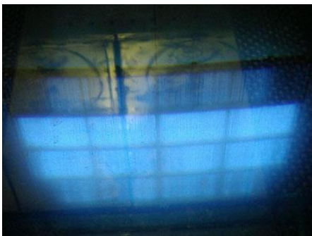
'Blue glow' from highly active Co-60 sources stored under water
